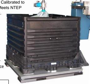
A single lance sub-surface foaming liquid filling system for 1 prestaged tote or IBC. Operator manually or automatically lowers lance into container. Fills to desired final net- weight.
